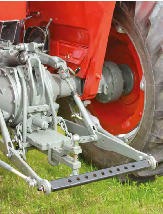
The drawbar has been modified over the years to better suit the rigours of working with the land-drive stone cart.
