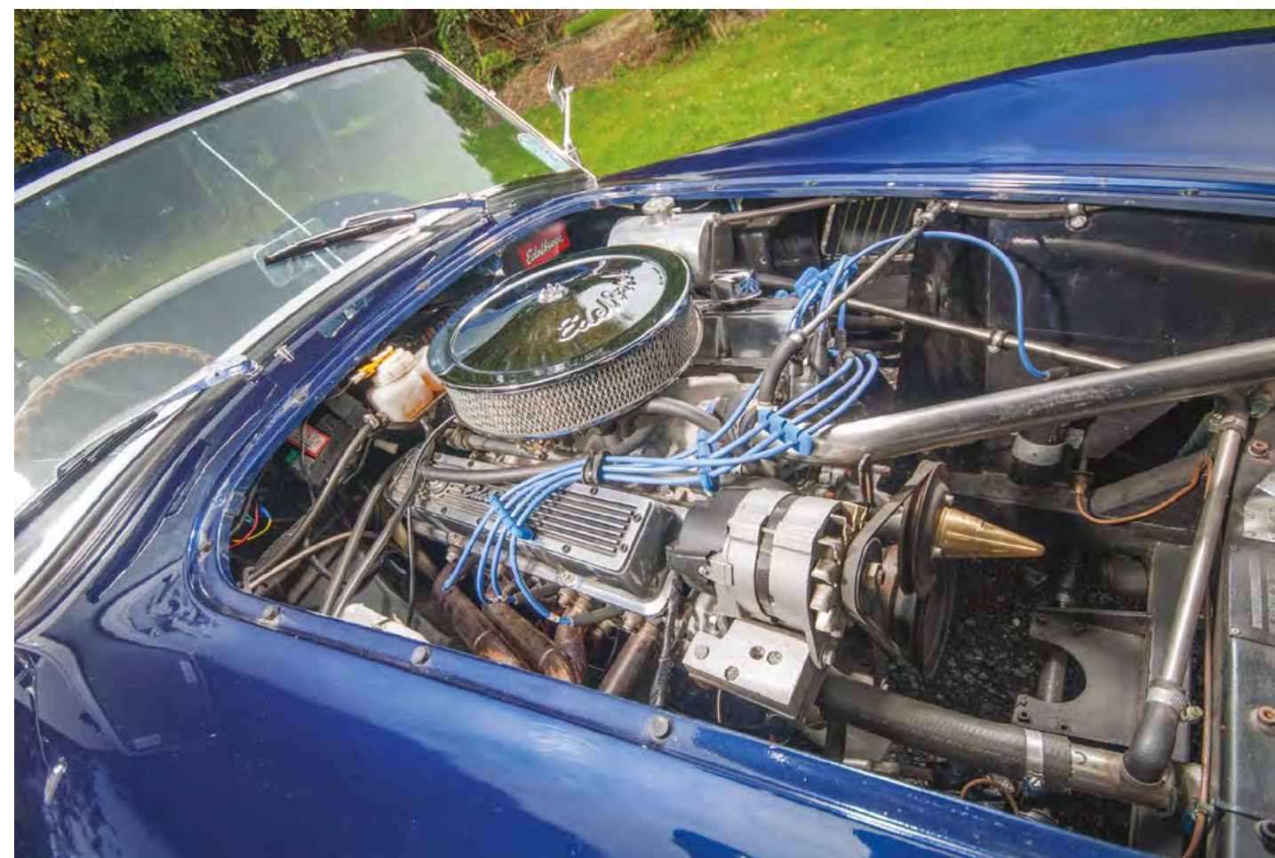
The Rover V8 fitted to Paddy's Cobra might "only" be a 3.5, but it's been well warmed up with a four-choke carb and manifold, electronic ignition and a hotter cam for north of 180bhp. Plenty of Edelbrock sparkle to be found too, with those eyecatching rocker covers and air filter. Note the tubular exhaust manifolds, which initially point forwards due to the constraints of the engine bay.
