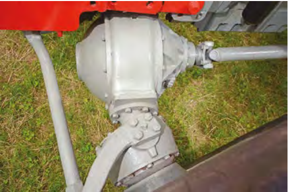
From the 'sandwich' transfer case by the gearbox, a propshaft delivers drive to the front axle.
