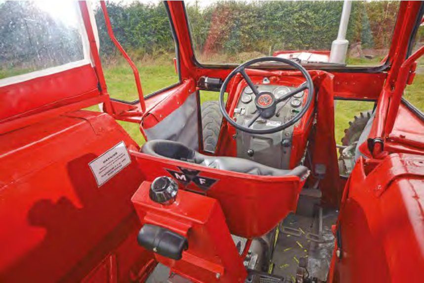
In the cab, you could almost be in a standard 178, until you look out of the windscreen, that is. Also, the extended transmission means that this cab is almost eight inches longer than usual.
