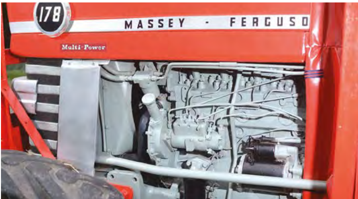
The four-cylinder Perkins diesel has been rebuilt several times in its working career, and it's estimated that it must have around 40,000 hours done.
