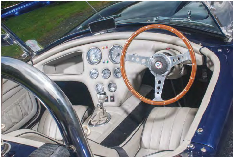
The grey leather interior has been well finished, which is just as well as it's on open show almost all of the time. The wiring loom kit used by the Dax utilises a Ford Sierra steering column, complete with its switches, which in turn acts on a steering rack from a Triumph Dolomite.
