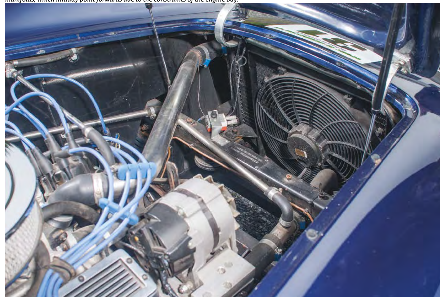
As it's smaller than the American V8s the Rover can be set well back in the frame for much-improved handling. You can see here how much room is left up front; the Jaguar V12 is also a popular engine choice for these Dax cars.
