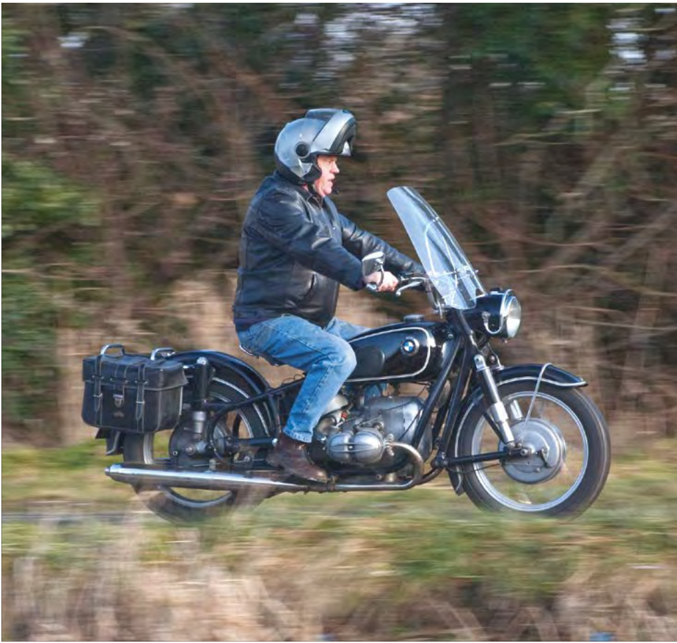
The large, polished casing at the front of the engine houses the highly durable electrics. Even though only 6-volt, the lighting is surprisingly good, we're told.
