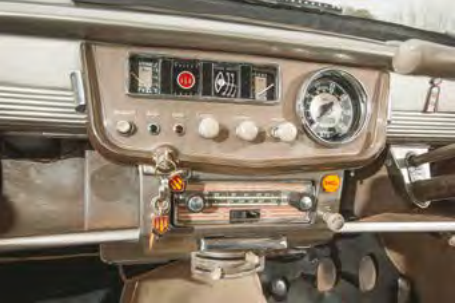
Stylish gauges and a lovely ‘Philips Transistorised’ radio inhabit the centre of the dash, plus a legend indicating the layout of the column-shifted gears.
