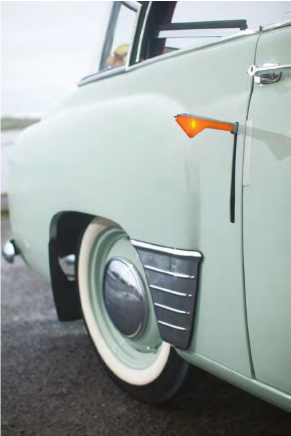
As there are no B-pillars (all of the side windows are retractable) the semaphore indicators had to be fitted in the rear quarter panels.
