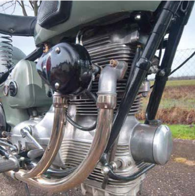
Inline two-cylinder OHC engine is fascinating, and very attractive thanks to those sweeping exhausts and teardrop air-cleaner; Brendan tells us the carb's proximity to the downpipes can lead to evaporation on occasion, one of the bike's few design flaws.
