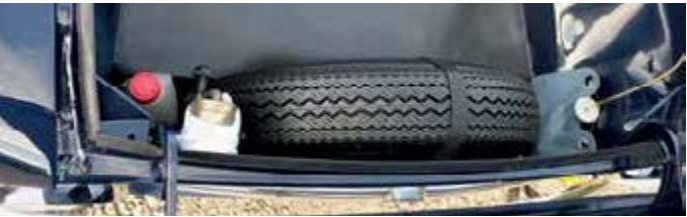
The boot up front, or "frunk" as it's apparently called now, is of a useful shape and size, and could easily swallow a few bags or shopping as well as housing the spare wheel and tool kit.
