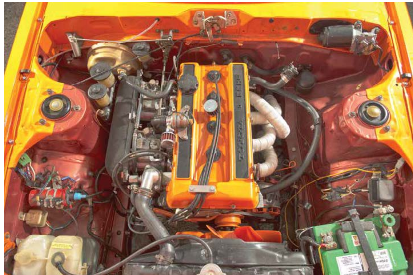
The 2000GT model was blessed with a 128bhp eight-valve two-litre twin-cam with dual twin Mikuni/Solex carbs. This one has only been mildly upgraded, but runs and sounds great.
