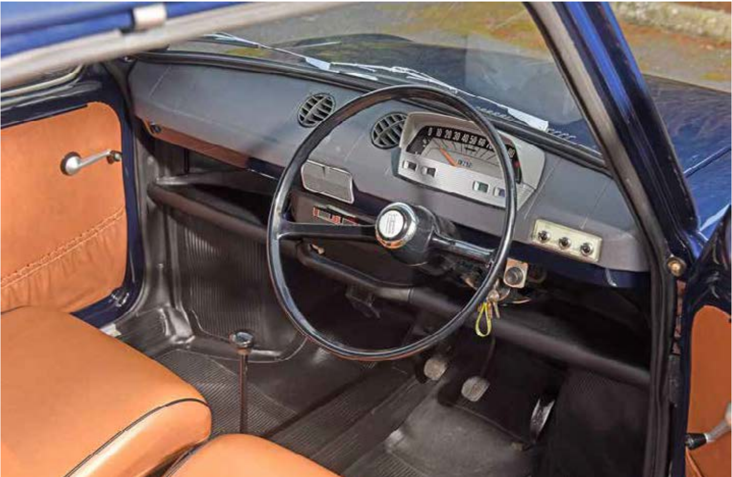
The interior is a master-class in stylish practicality. Note the durable rubber floor covering, single instrument binnacle and slim, lightweight seats. It's deceptively roomy in there too.
