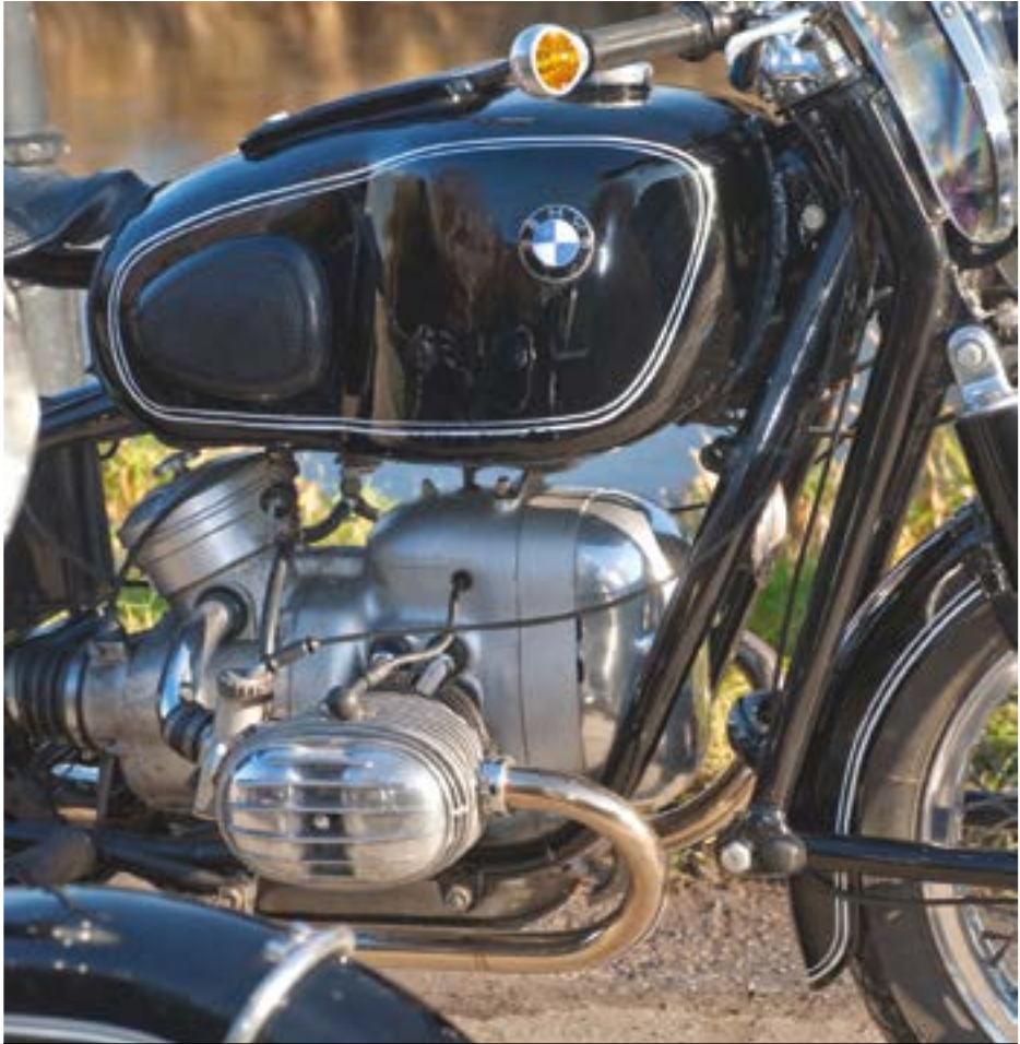
The large, polished casing at the front of the engine houses the highly durable electrics. Even though only 6-volt, the lighting is surprisingly good, we're told.
