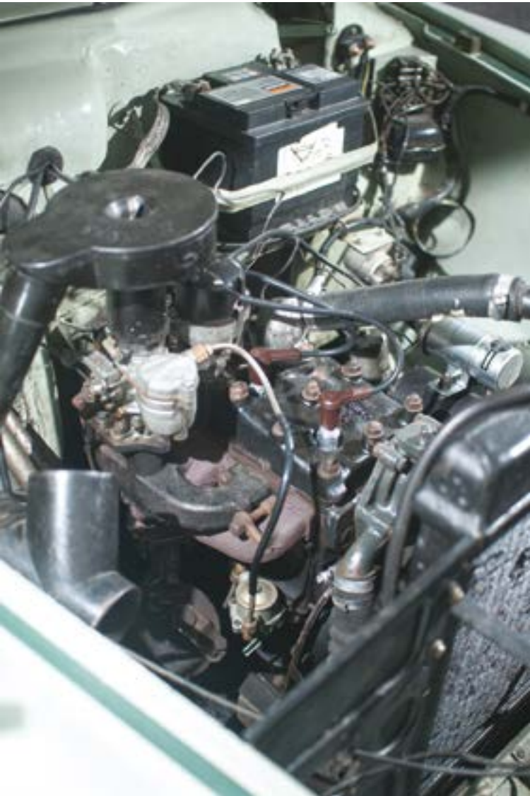
As this is an early 1954 model it features the 1,265cc sidevalve engine, which was replaced by an OHV 1,390cc later on that year.
