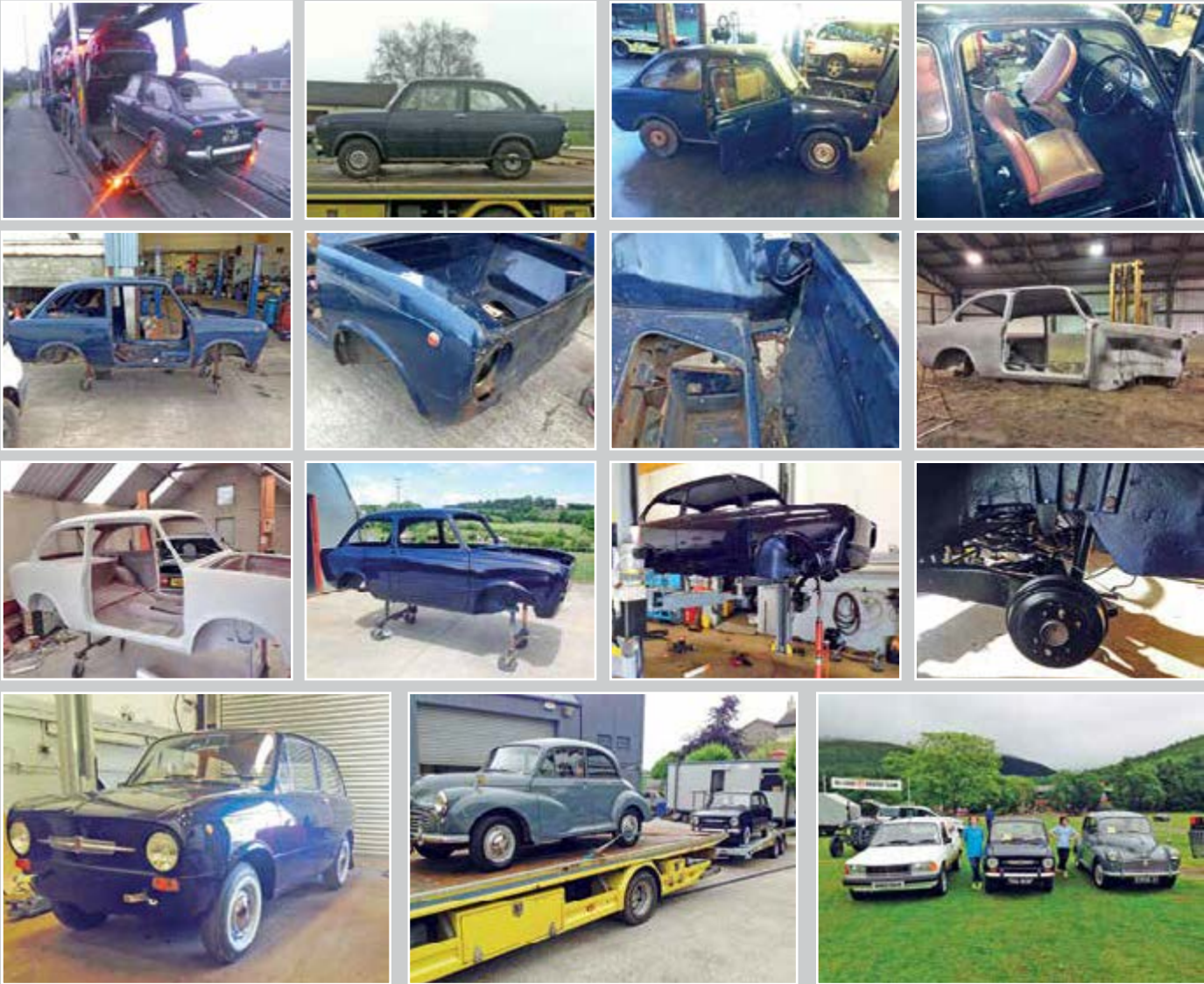
All of Eunan's mechanical skills were called into action during this project. The first four images show the Fiat as it arrived off the transporter from the UK to his home in Banbridge, untouched for many years and in extremely original condition overall. Unfortunately the strip-down uncovered some rot, particularly in the nose and boot floor, and a thorough sand-blasting soon revealed all. However Eunan was
