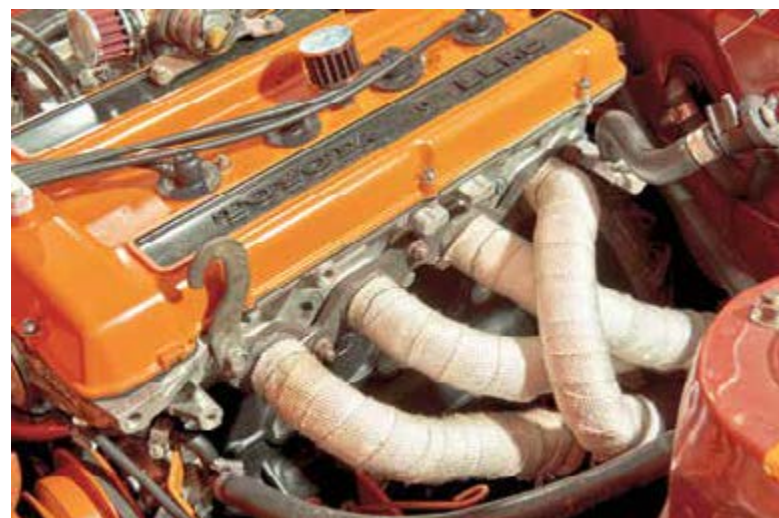
Heat-wrapped four-branch manifold frees a few extra horsies.
