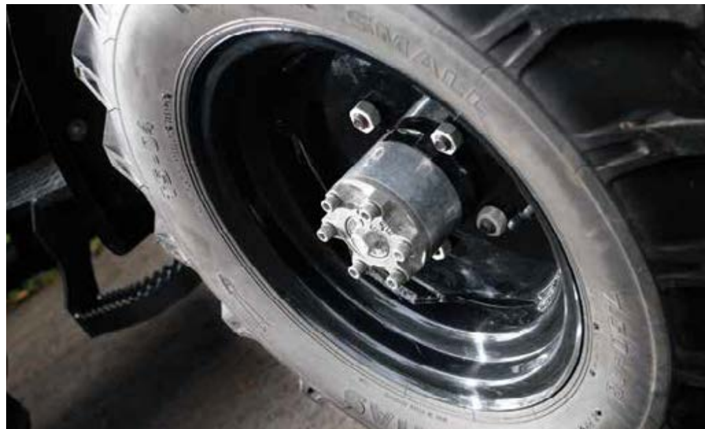
Front hubs are freewheeling items adapted from their usual Land Rover application.
