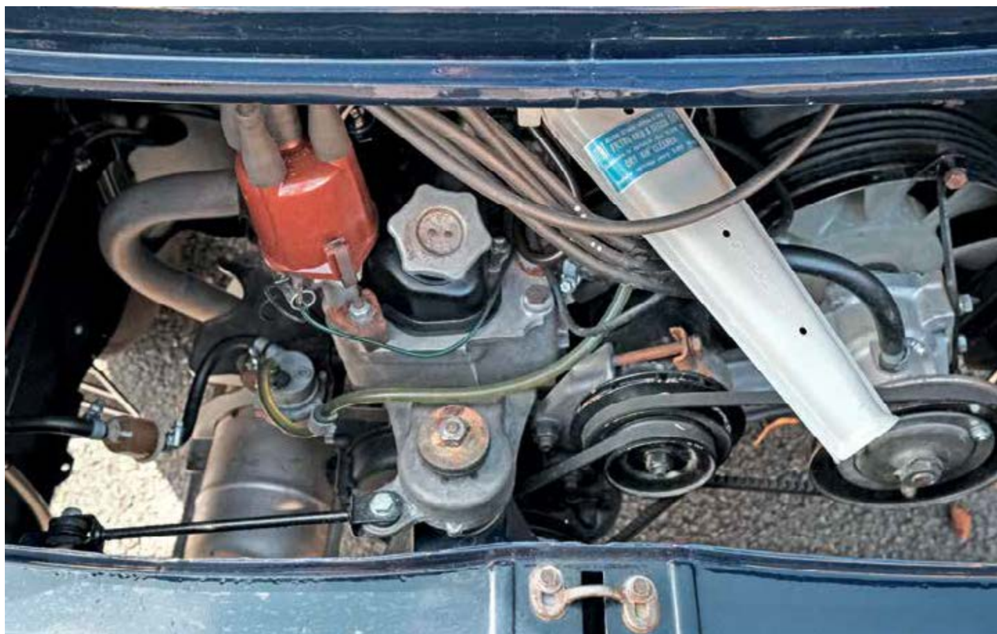
The four-cylinder, 843cc engine is water-cooled by a radiator mounted alongside, cooled by the fan visible on the upper right here. Given adequate maintenance it runs coolly and reliably.
