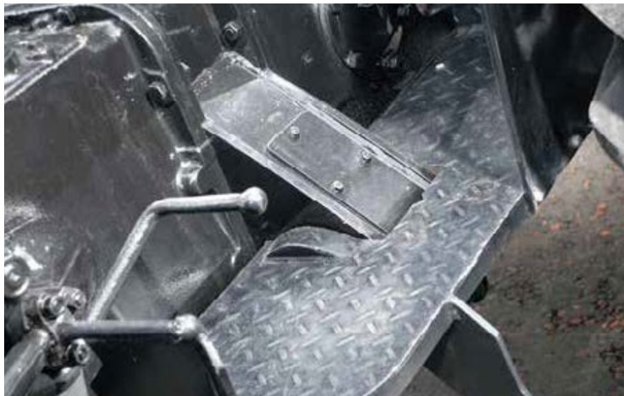
There's a lot of neat fabrication in this shot alone; the adapter plate sandwiched between the gearbox and axle looks almost standard, and a tidy inspection plate has been incorporated into the chain cover.
