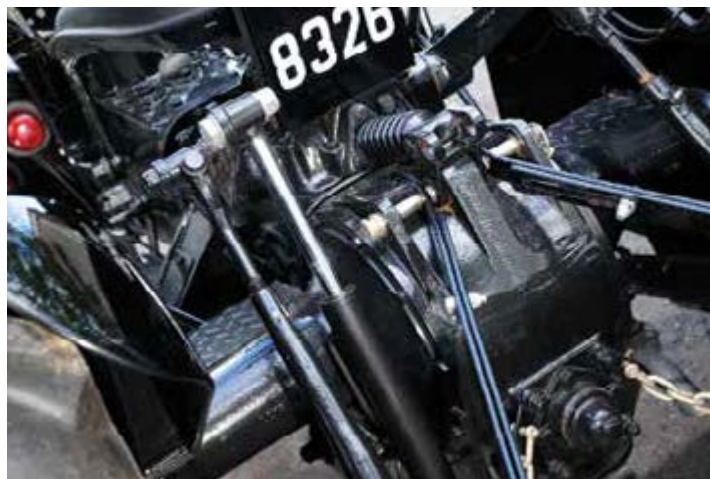
Hefty extra ram augments the usual hydraulic system at the rear.
