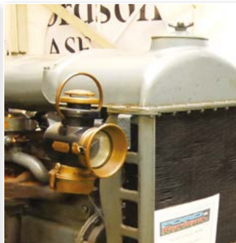
Check out these great, period-correct acetylene lamps fitted to Bernard O'Gorman's 1918 Fordson MOM.
