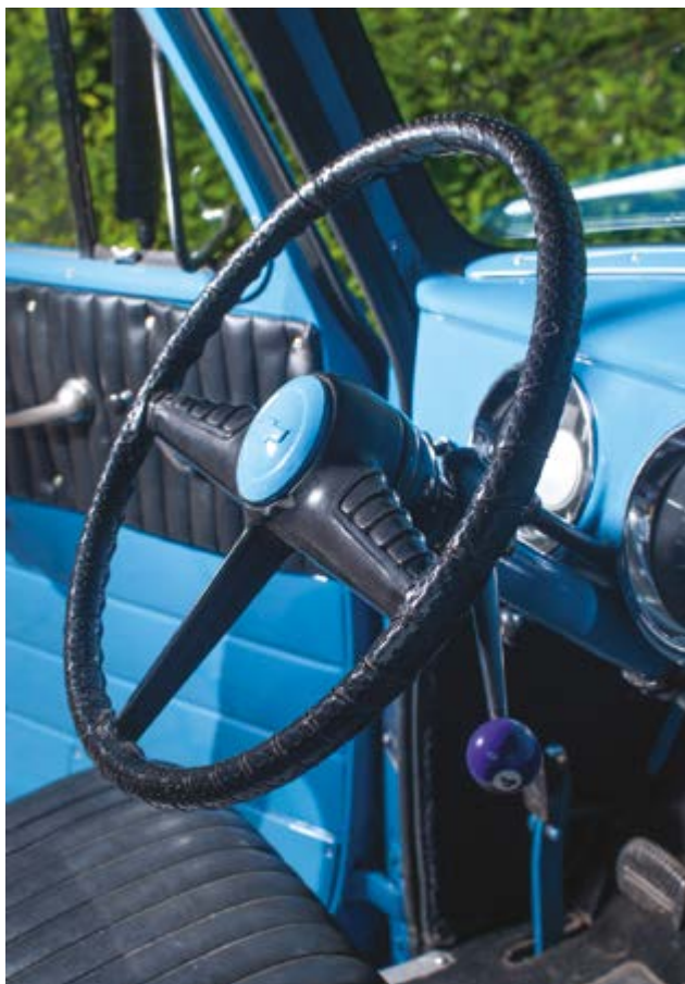
The three-speed manual has a column-shift, or as the Americans would say, "a three on the tree".
