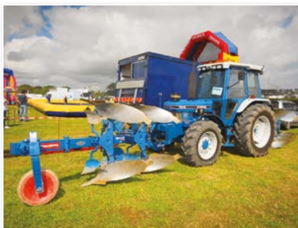
The Ford 7610 of Michael Hoey, which is fitted with impressive reversible Ransomes ploughs front and rear. The operation of this 'push/pull' machine was demonstrated by John Baggaley throughout the event.
