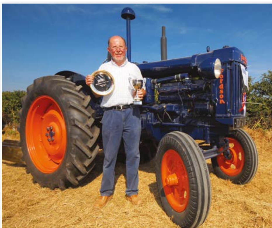
John Daly with his winning Major, which is a 1947 model with a 1950 Perkins P6 conversion and Ransomes 3-furrow plough. The stunning machine is a worthy winner; well done to John.
