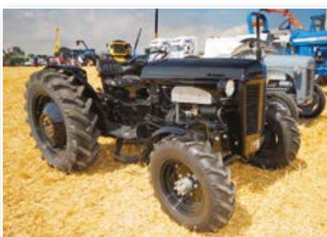
G. Marmion's Ferguson 20 stood out for 3 reasons: it's black, it has a Land-Rover based 4wd conversion, and it is utterly stunning in every detail.
