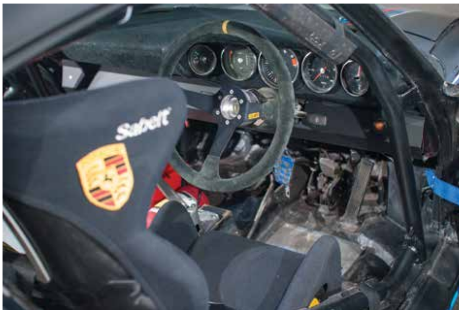
Like most race cars, the cockpit isn't built for looks, but business. Note the modified clutch pedal for easier heel-and-toe action.
