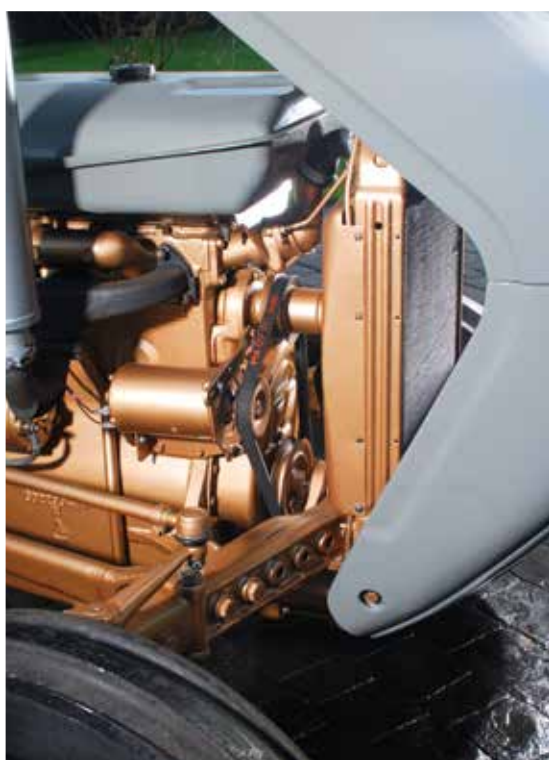
The original radiator was re-cored during the restoration, and all other ancillary items were either rebuilt or replaced.
