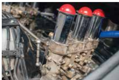
Triple-choke Webers are a 911 peculiarity, and sound amazing.
