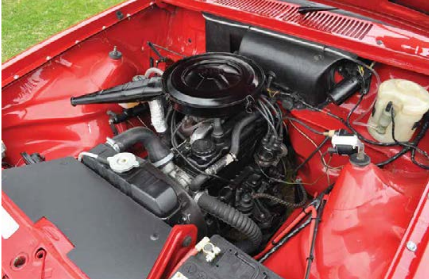
The 1.2-litre OHV Opel engine is known for its reliability and decent performance, and this one lived up to that, with the bottom end needing no work during the restoration.
