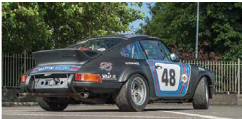
The rear end features a 2.7 RS-style ducktail engine cover, custom exhaust and plenty of "speed holes".
