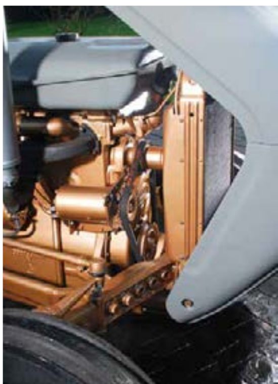
The original radiator was re-cored during the restoration, and all other ancillary items were either rebuilt or replaced.
