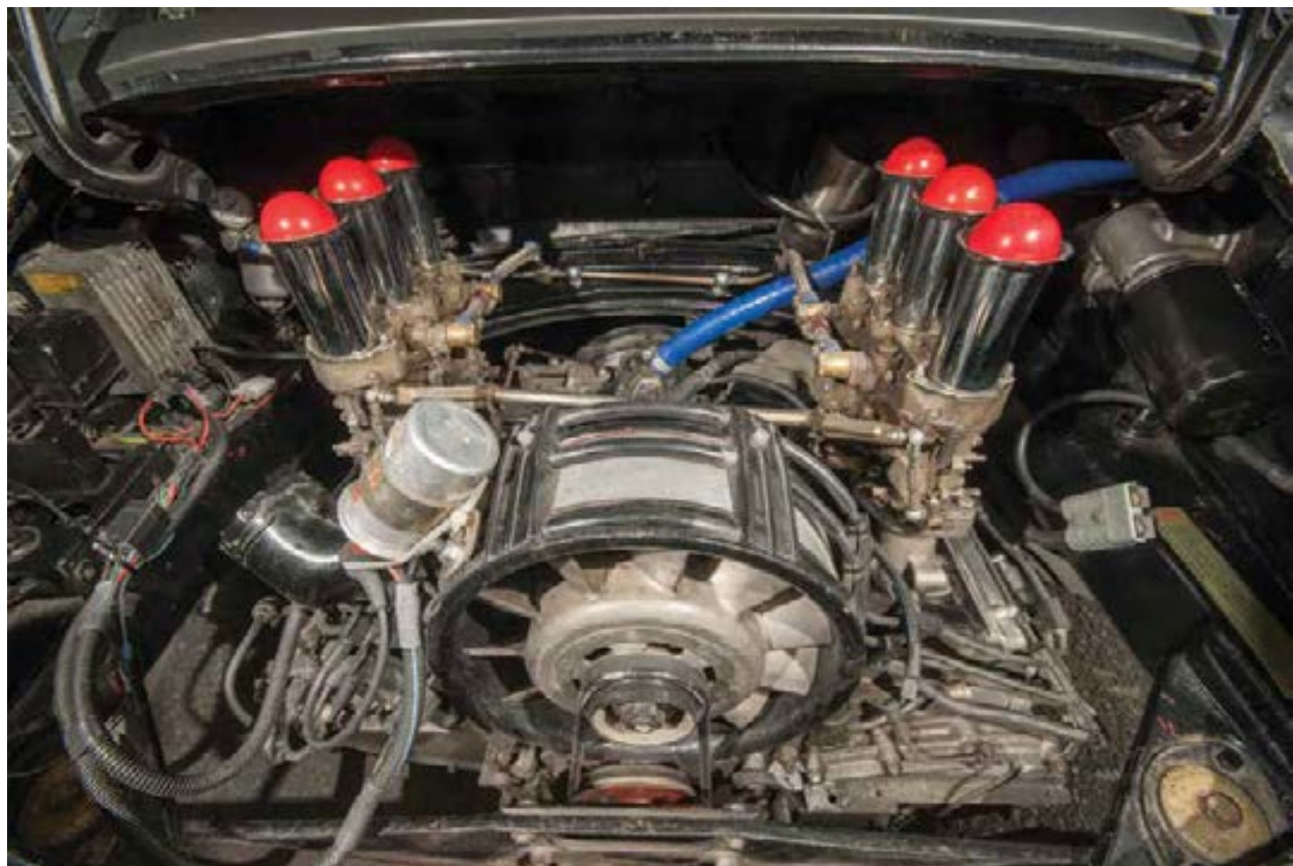
In place of the two-litre motor that would have been in the base car, this racer now sports a 280bhp 2.7-litre powerhouse.
