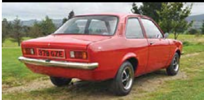
Note the fuel filler hidden under a hinged panel on the C-pillar.
