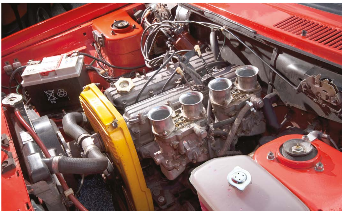
The Abarth's twin-carbed 2.0 16v DOHC was more highly strung then the Sport; this one even more so thanks to those open chokes.
