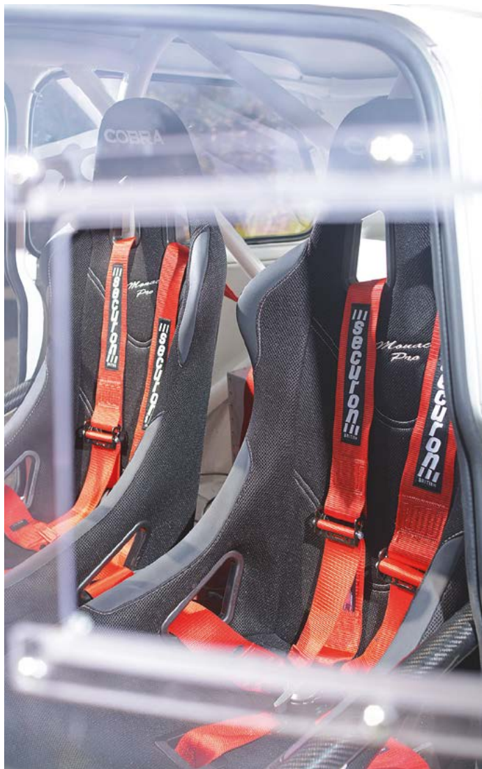
Polycarbonate windows, full cage, harnesses and buckets – no concession to luxury here.
