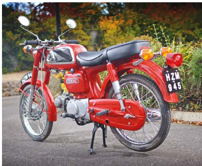
Enclosed chain and large mudguards don't take from the S90's sporty looks. Note the T-shape of the pressed steel frame.
