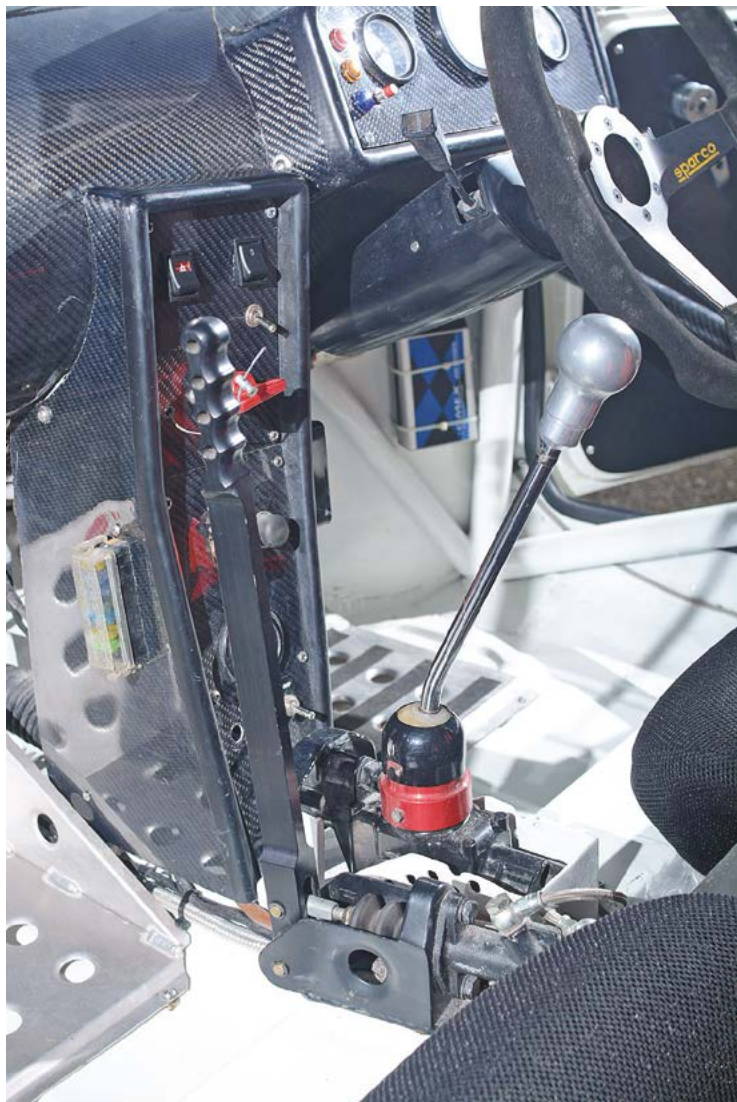
External gear selector and hydraulic handbrake are neatly to hand. The carbon-fibre dash holds the bare necessities and nothing else.
