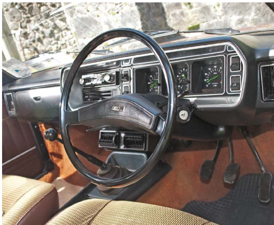
The interior of Robert O'Shea's Series 1 1600 Special shows how well-specced it was in 1976, with a five-speed 'box, rev counter and radio/cassette just some of the goodies.
