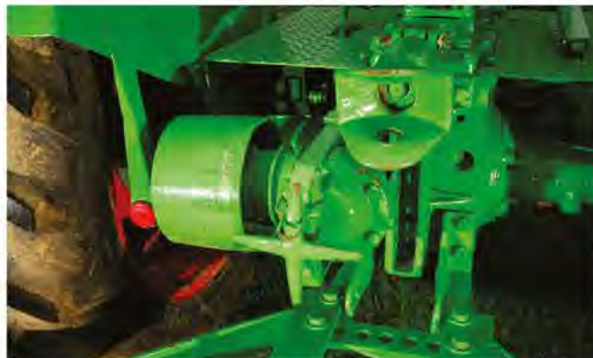
Belt pulley is easily removable to gain access to PTO.
