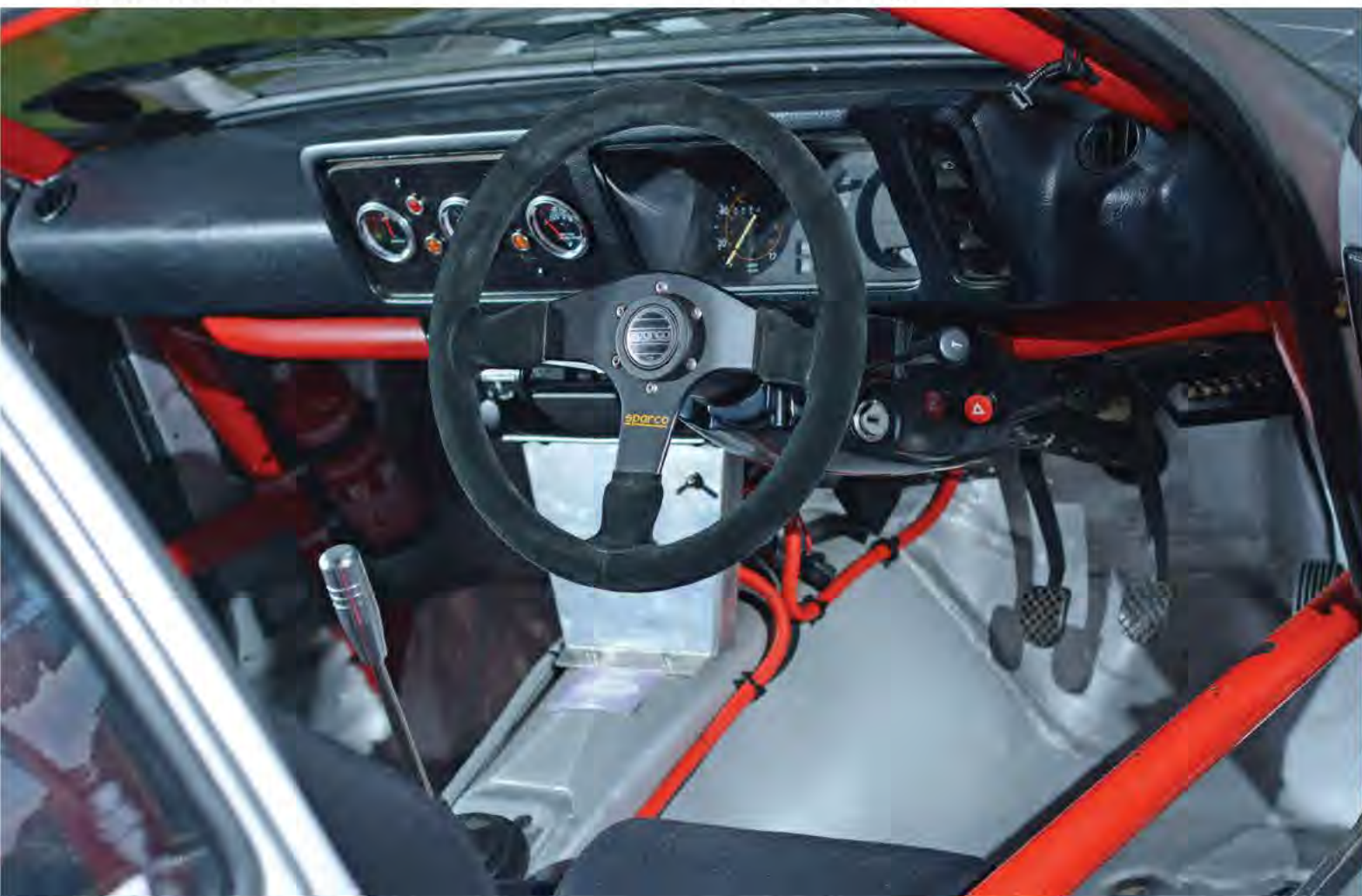
The cockpit is all business – Des wanted this to sound and reel like a rally car, and he's really succeeded in that. There isn't even a headlining in there, and the impressive cage runs under the dash and out to the front suspension too.
