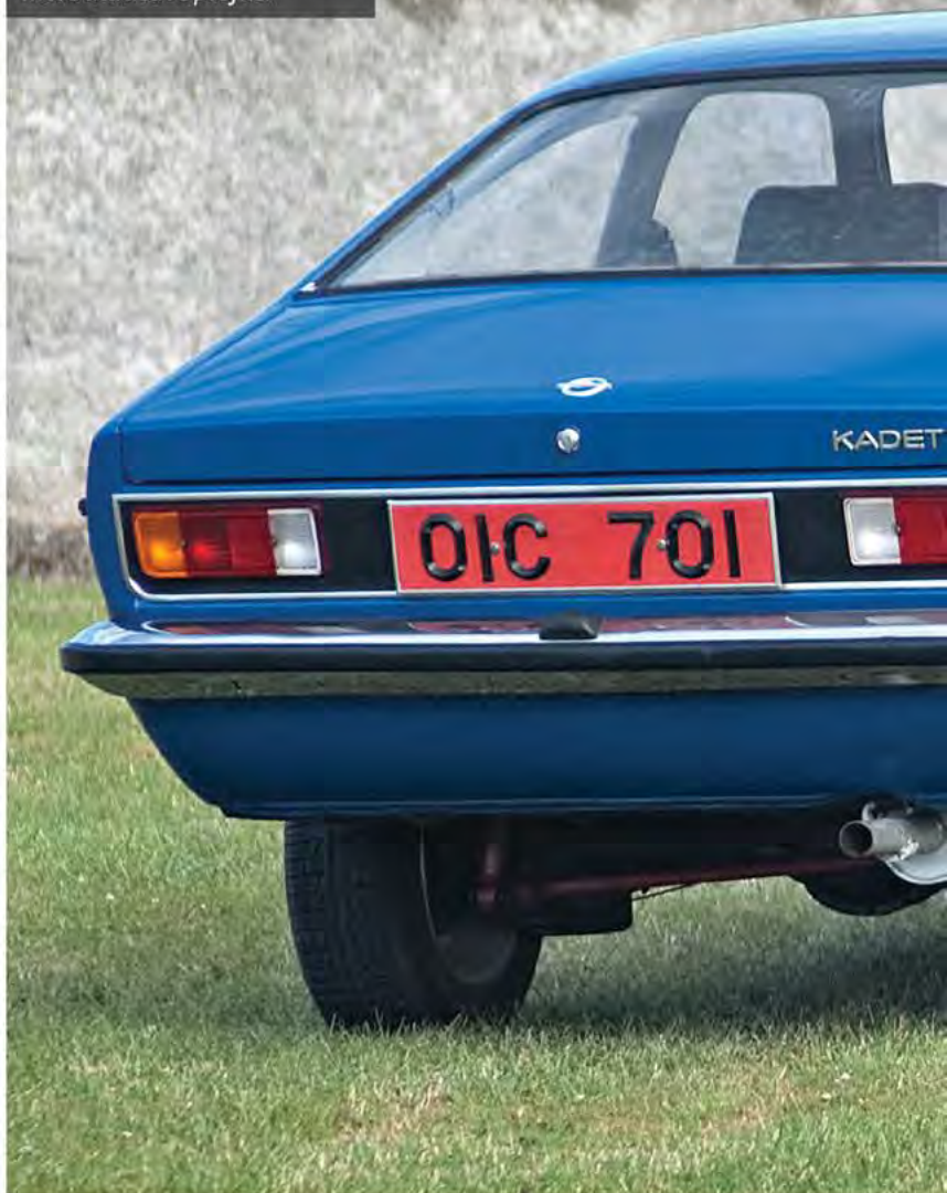
Even the original bumpers have survived in excellent order. Frank has rustproofed and painted their inner surfaces to preserve them for the next thirty years.
