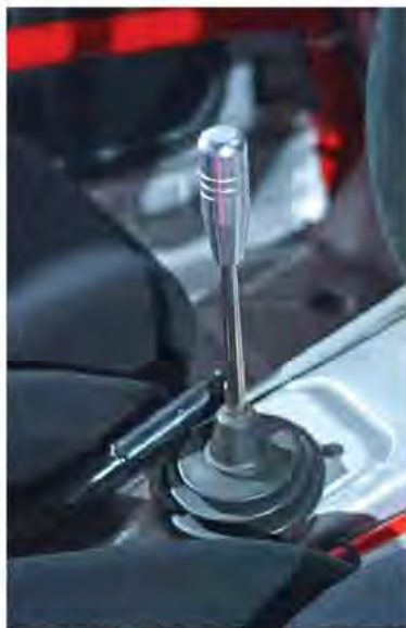
The elegant alloy shifter stirs a Ford Type-9 gearbox.
