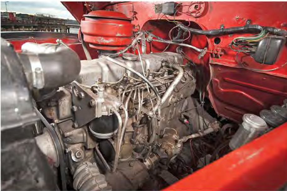
The big six-cylinder Perkins 6354 is a familiar beast to Billy, as it was used in many industrial and marine applications. This one replaced the original six-cylinder petrol at some stage in the truck's past, but runs nicely after some remedial work was performed.
