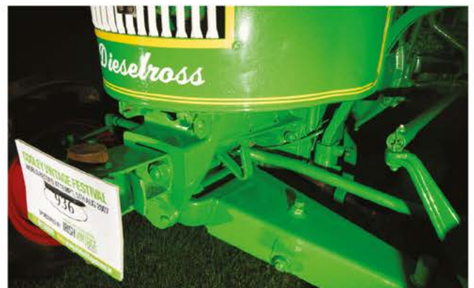
Ingenious split front axle is leaf-suspended.
