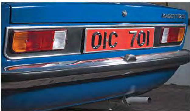
Even the original bumpers have survived in excellent order. Frank has rustproofed and painted their inner surfaces to preserve them for the next thirty years.
