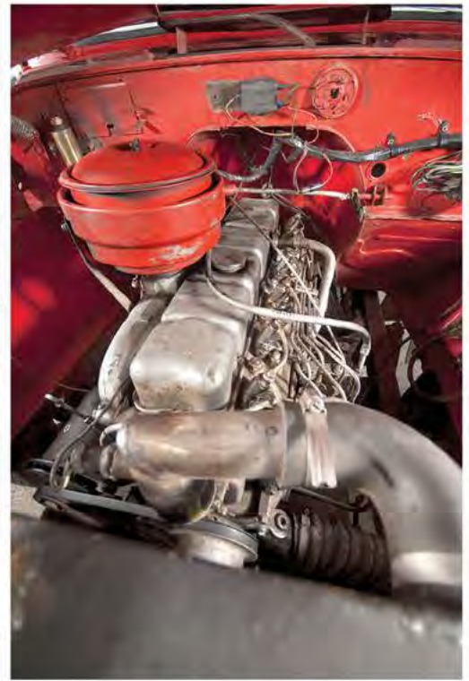
The big six-cylinder Perkins 6354 is a familiar beast to Billy, as it was used in many industrial and marine applications. This one replaced the original six-cylinder petrol at some stage in the truck's past, but runs nicely after some remedial work was performed.
