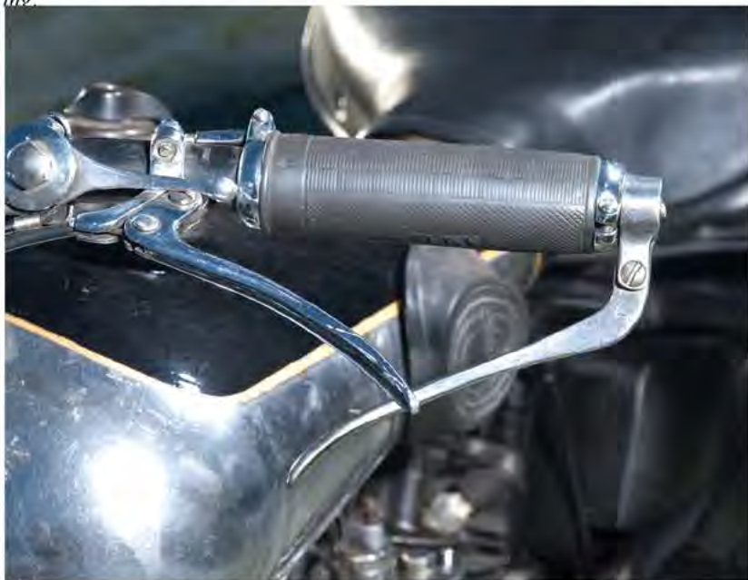
Handlebars feature both conventional and inverted handles. Both sides feature twist grips, one for the throttle and one for the advance/retard mechanism.
