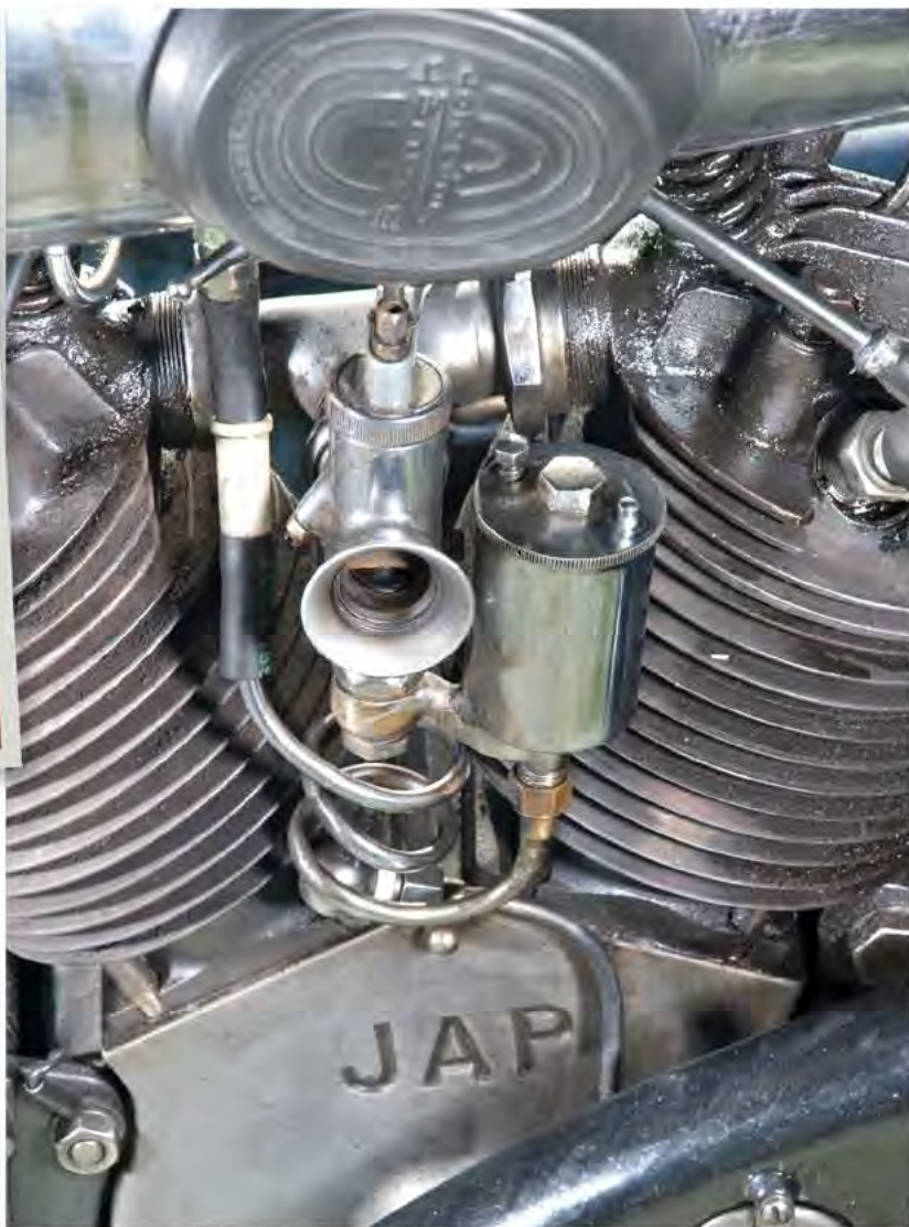
Both barrels of the V-twin are fed by an Amal 1.125-inch carburettor. This bike's reliability is such that Paddy tells us he never needs to use the choke when starting.
