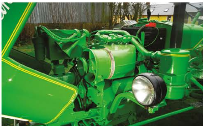
Twin-cylinder diesel is dominated by the cooling fan and ducting.
