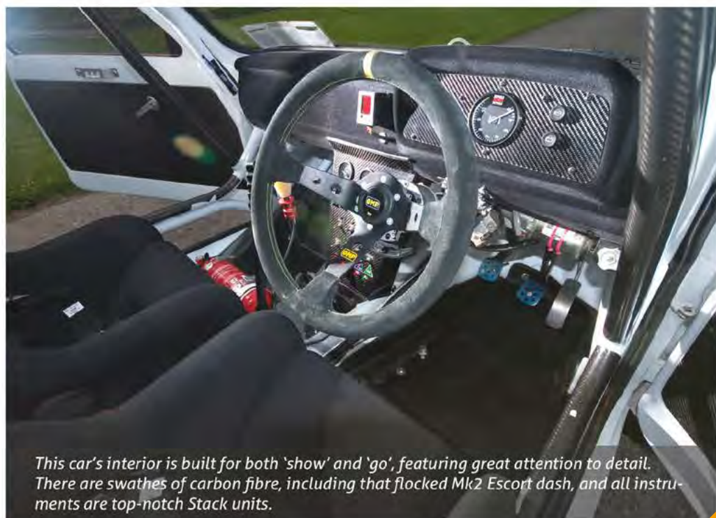
Hydraulic handbrake, sequential gear shifter and steering column switch are mounted together at the same height for quick response. Note the extent of the roll-cage tubing on the left.
