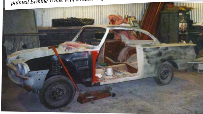
At an advanced stage of the project, with the body structure back in one piece.
