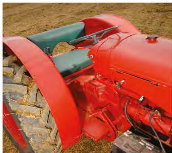
Bench seat and right-hand clutch and brake pedals were to facilitate the carriage of a passenger.
