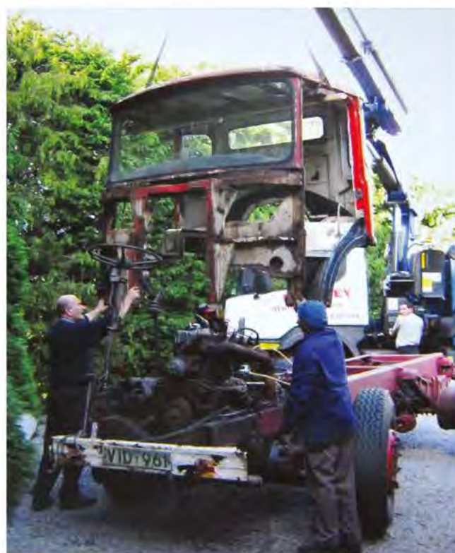
The repaired cab structure being reunited with the primed chassis.
