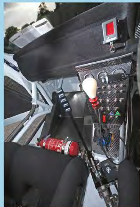
Hydraulic handbrake, sequential gear shifter and steering column switch are mounted together at the same height for quick response. Note the extent of the roll-cage tubing on the left.
