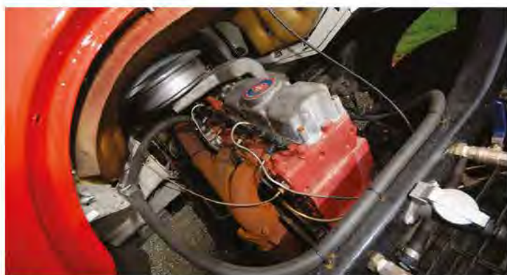
AEC straight-six was a well-proven unit, and has proven its toughness in this application as it hardly needed to be touched during the project.
