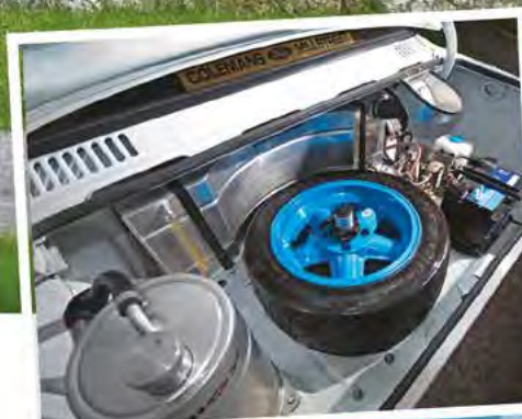
Boot installation was completed with the same care as the rest of the car. The dry-sump oil tank is mounted on the left, while the twin Facet fuel pumps and battery circuitry are on the right.
