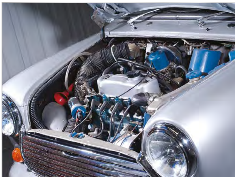
The old 850 engine is long gone, with a warmed-up 1275 in its place. It features a K&N filter, Lucas competition coil and leads and plenty of detailing.
