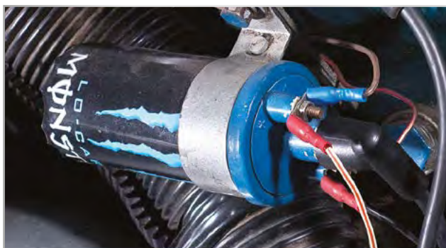
The old 850 engine is long gone, with a warmed-up 1275 in its place. It features a K&N filter, Lucas competition coil and leads and plenty of detailing.
