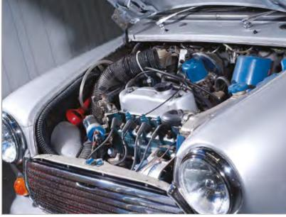
The old 850 engine is long gone, with a warmed-up 1275 in its place. It features a K&N filter, Lucas competition coil and leads and plenty of detailing.
