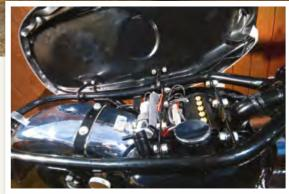
The under-saddle area is as well-detailed as the rest of the machine, and features many hand-fabricated items. Gary has fitted a new wiring loom with a modern regulator, but has also kept the originals in situ so they can be easily reinstated if desired.
