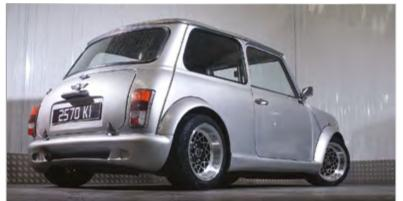
The spaced rear wheels and adjustable suspension give this Mini a very purposeful stance.
