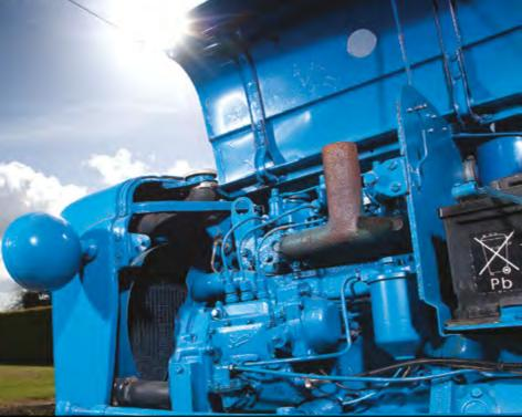
Having received new internals and a new cylinder head this three-pot Perkins runs as sweet as a nut, and starts after barely a turn.
