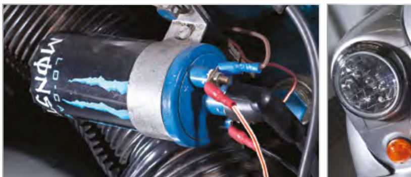
The old 850 engine is long gone, with a warmed-up 1275 in its place. It features a K&N filter, Lucas competition coil and leads and plenty of detailing.
