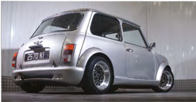
The spaced rear wheels and adjustable suspension give this Mini a very purposeful stance.
